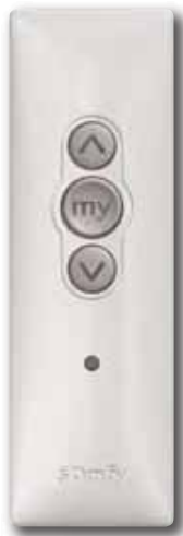
Situio RTS Room control. To control a single window covering.
