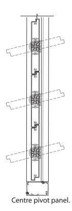
**Note:** When rear pivot panels are over 2000mm in blade span, a connecting rod is required.
